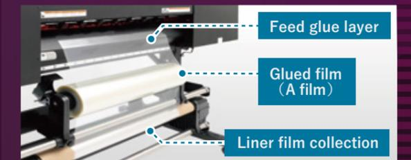
Automatically takes-up the UV-DTF film liner paper at the back of the machine. The liner paper is rolled precisely at the printer's feeding speed, ensuring stable printing.
