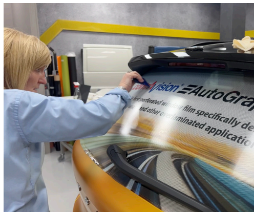
AutoGraph features air release channels within the adhesive.
