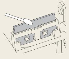
Dirt around the wipers may lower the effect of the automatic cleaning and can also be a factor of damaging the print heads.
