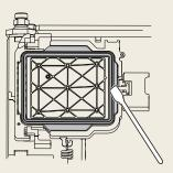
The accumulation of dirt around the cap gasket impairs the print head's seal to the cap. Over time, this problem can cause premature print head failure.
