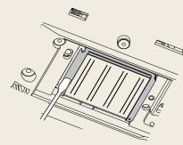
When dirt accumulates along the sides of the print head, print quality is impaired. This can also cause a premature print head failure
