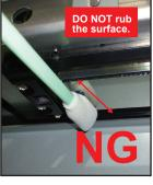
Rough cleaning may damage the print head's water-repellent coating and worsen the problem.
