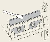
Dirt around the wipers may lower the effect of the automatic cleaning and can also be a factor of damaging the print heads.
