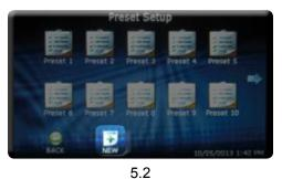
Press the NEW button on the preset setup screen. (5.2)
