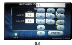
Using the displayed Keyboard/ Keypad, enter the numeric time values and press ENTER. (8.5)
